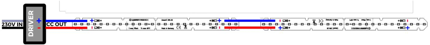
The series connection is applied by connecting the positive (+) terminal of the first LED strip to the negative (-) terminal of the second LED strip. This pattern is repeated for further LED strips, from the negative (-) of the second strip to the positive (+) of the third strip and so on. At the same time, the negative (-) of the first LED strip is wired to the (+) of the second, then the (-) of the second to the (+) of the third and so on.
